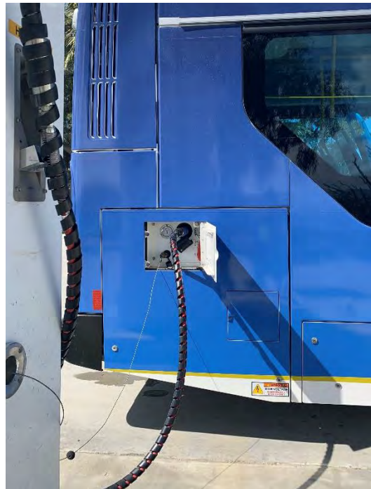
Photo 2: Fuel Cell Energy Bus Refueling
