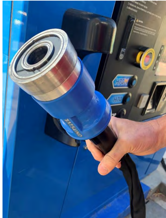
Photo 1: Hydrogen Fuel Pump Station
