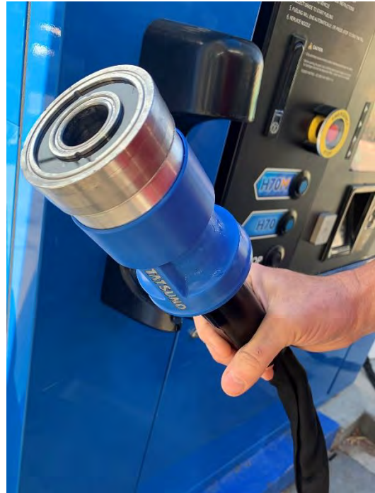
Photo 1: Hydrogen Fuel Pump Station
