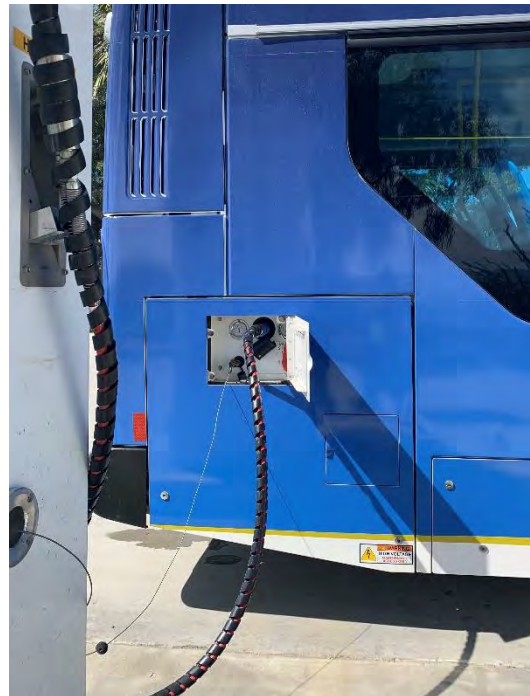
Photo 2: Fuel Cell Energy Bus Refueling
