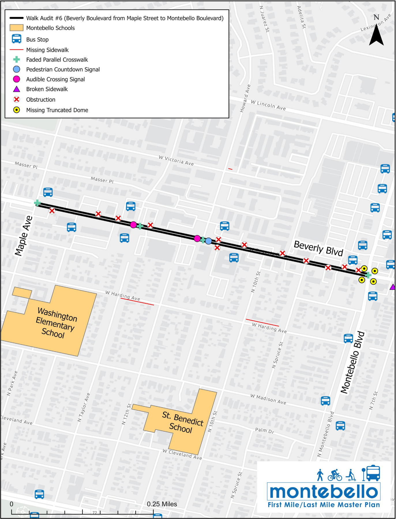
FIGURE 2-19: Existing Conditions along Walk Audit #6 Route
