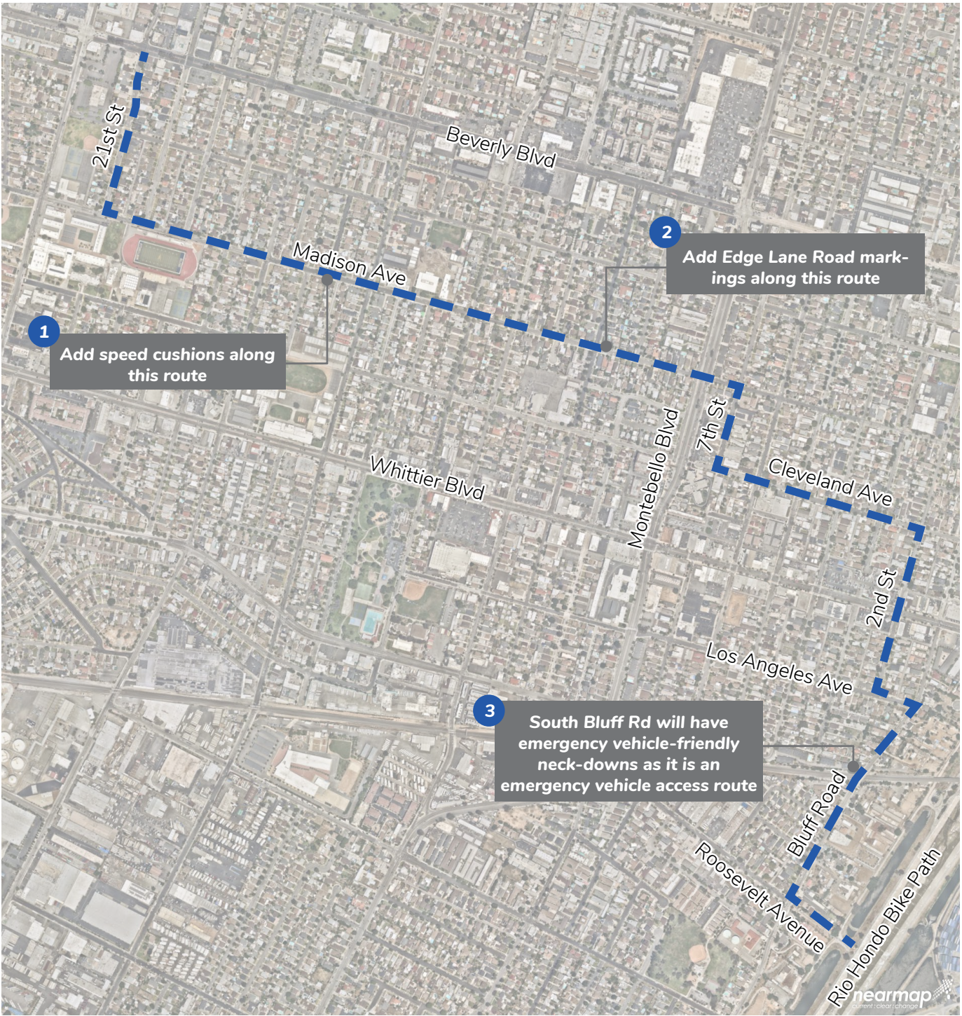
FIGURE 6-9: Neighborway with Edge Lane Road Markings and Speed Cushions
