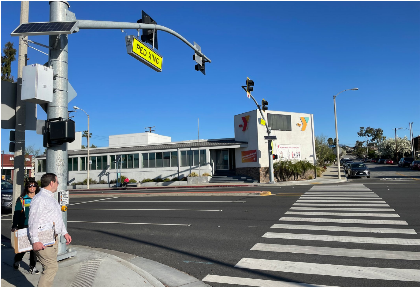
A Pedestrian Hybrid Beacon (PHB) at Beverly Boulevard and 20th Street
