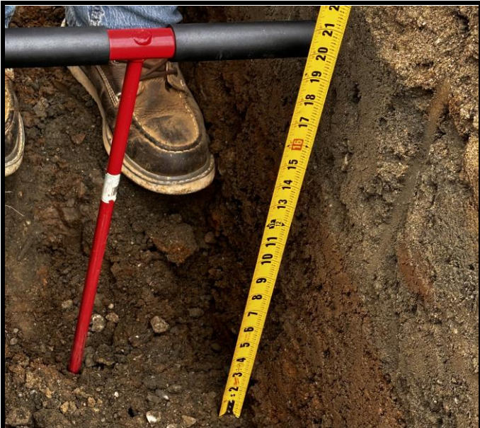
Probing at 16 inches when chasing saturated soil
