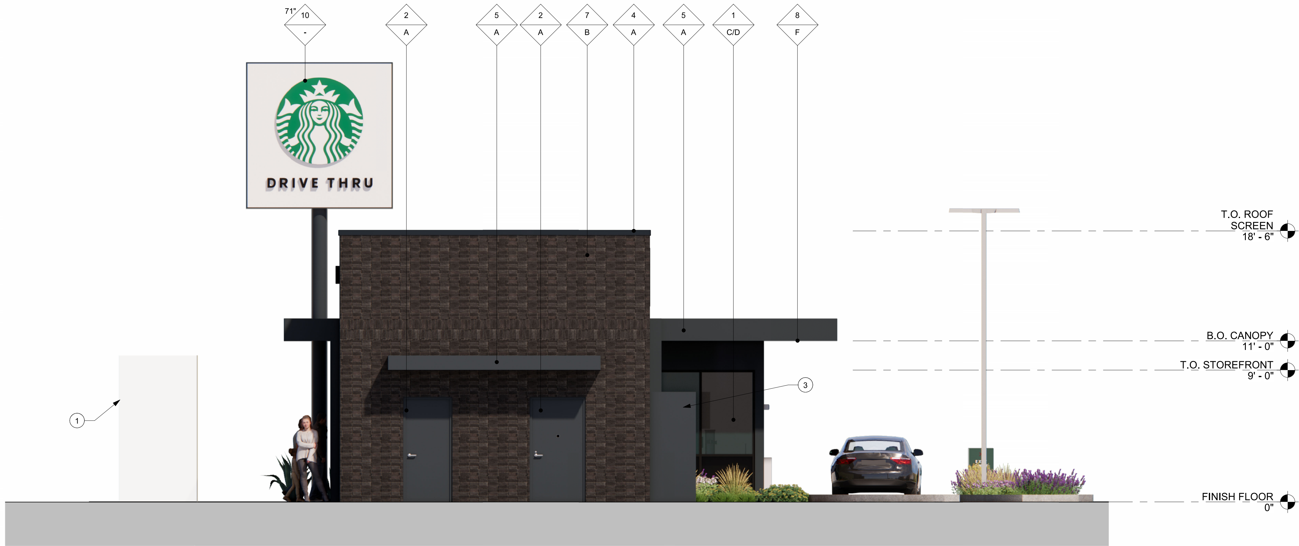
2 PROPOSED COLOR WEST ELEVATION Scale: 1/4" = 1'-0"
