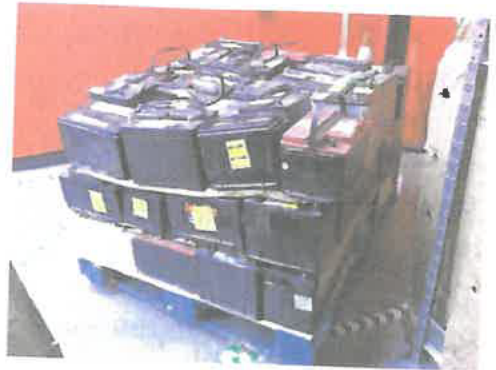
Pallet of scrap lead-acid automotive batteries ready to be recycled
